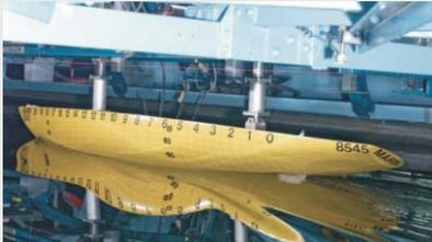
Captive basin tests for hydrodynamic loads with heel, leeway and rudder in the Deep Water Basin
