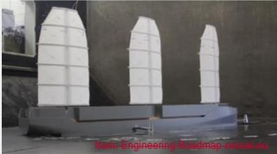
Subcontracted wind tunnel tests to verify aerodynamic performance
